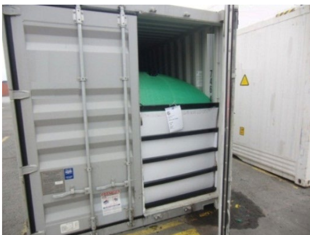
Figure 7.51 Container fitted with flexitank
