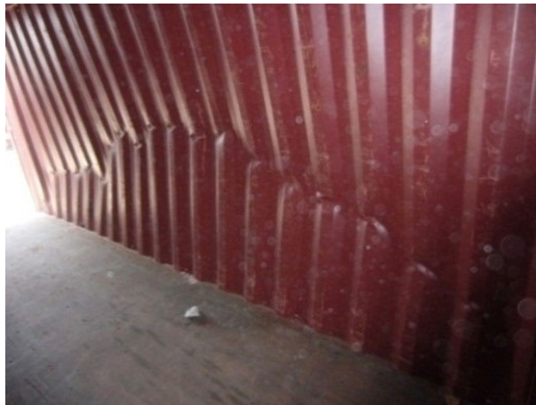
Figure 7.50 Damaged CTU side wall
