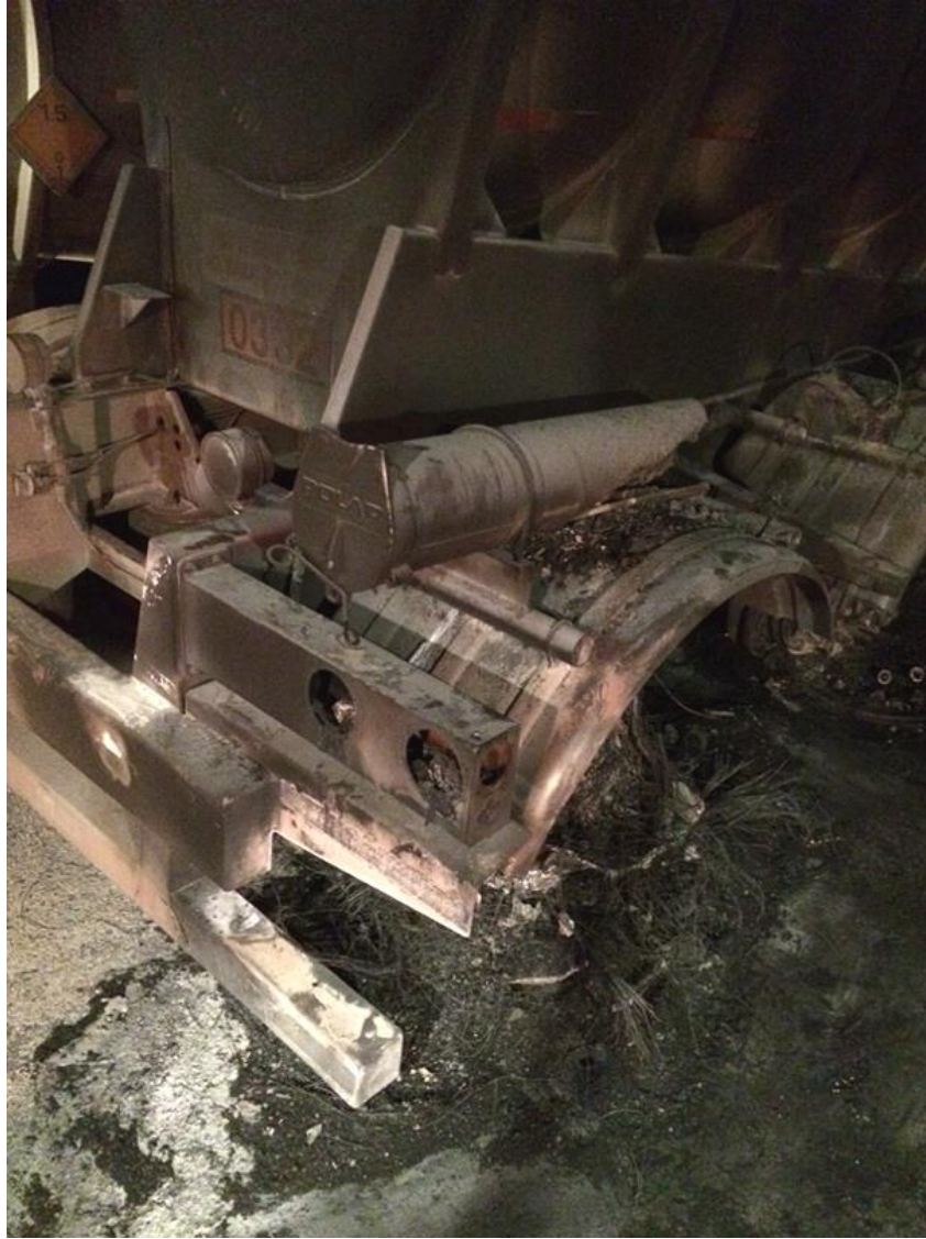
Figure 6: Burnt and melted tire area
