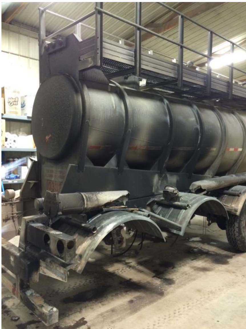
Figure 5: Tanker in the workshop showing heated-affected areas
