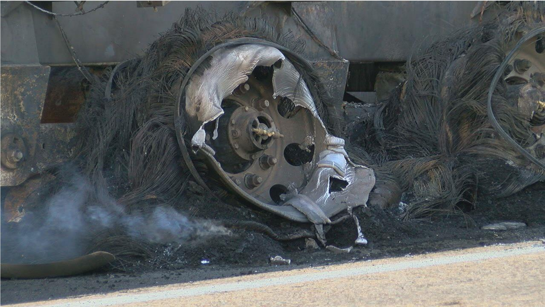
Figure 2. Closeup on the burnt tire area
