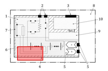
5. The safety system that is part of high voltage batteries is designed to protect against an external short-circuit. As a result, test is passed without current flow, because the protective components, (red shaded box in illustration 6) are preventing it, via a fast reaction-rate open-circuit disconnect. This is the best technical way to prevent the risks related to the application of an external short circuit.
