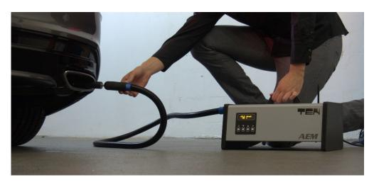
• Instrument : Particle counter with spec's according to NPTI-working group
