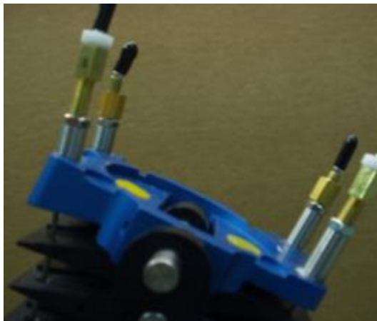
Figure 49 Damper cable adjusters
