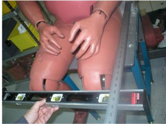
Figure 10 Measuring the seated height of the dummy
