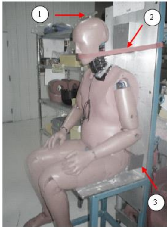
1. Head Level Tool. 2. Head Strap. 3. H-Point Tool (App.9/Dwg.004)
