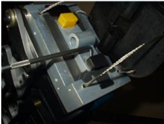
Figure 84 Using a pick to remove the T1 bumper
