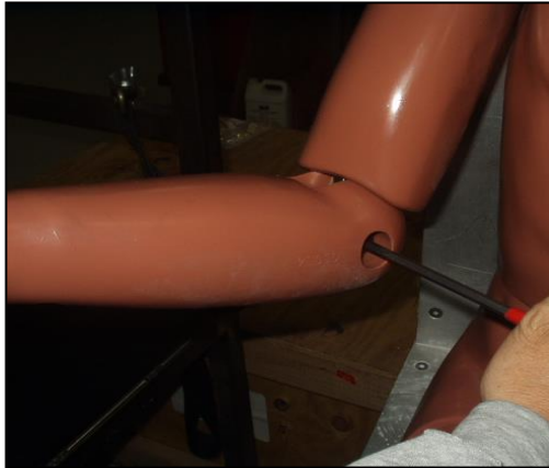
Figure 62 Adjusting the elbow pivot bolt
