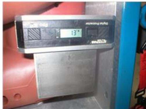
Figure 6 Measuring the H-point tool angle
