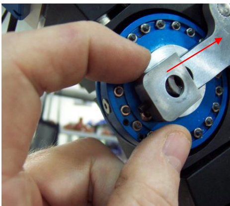
Figure 12 Install Damper Clamp Bracket
