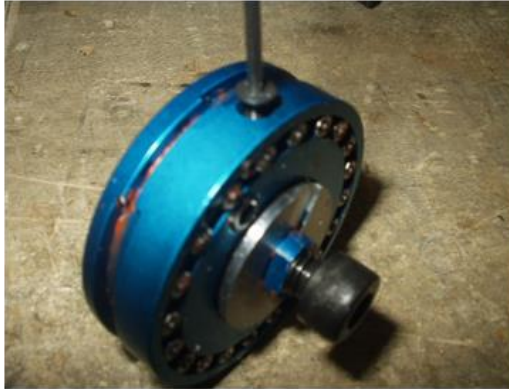
Figure 33 Remove Oil Fill Screw
