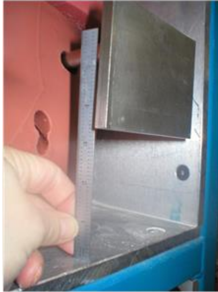
Figure 6 Measuring the H-point tool angle
