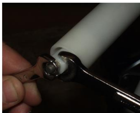
Figure 43 Lock the Spring Cable Adjusters
