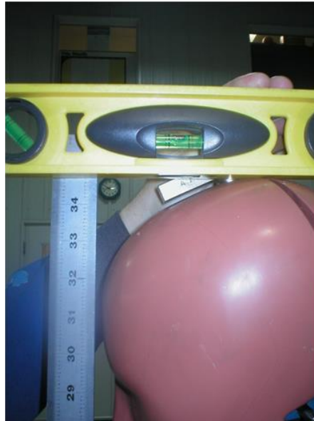
Figure 11 Measuring the left knee pivot height
