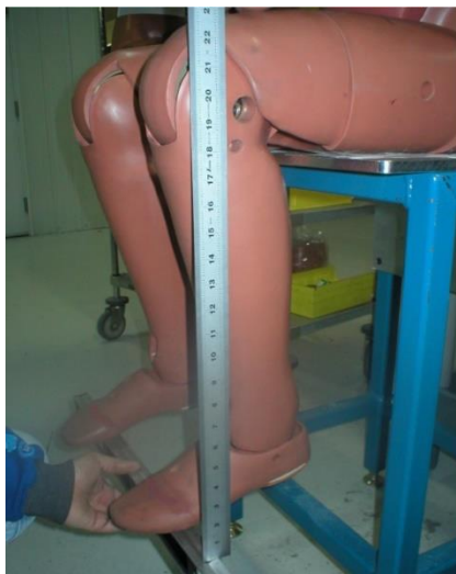
Figure 11 Measuring the left knee pivot height
