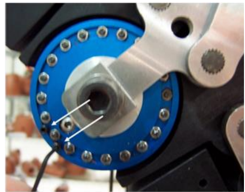
Figure 27 Loosen M3 Clamping Screws
