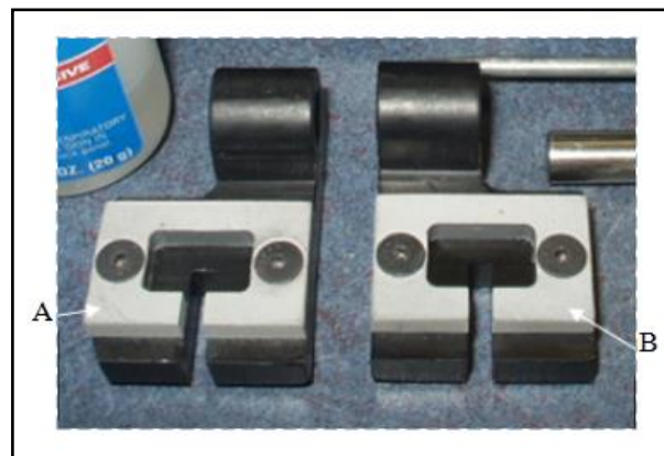
Figure 80 Cervical Bumper Installation Tools. A, for C2, C4 and C6; B, for C3, C5 and C7
