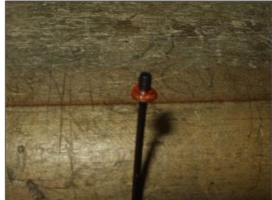
Figure 34 Add sealant to the cover screw
