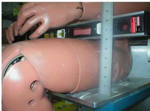
Figure 8 Measuring the thigh clearance
