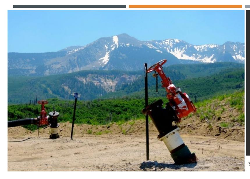
Well heads on gob vent boreholes above the West Elk Mine in western Colorado. It is 4Mtpa automated longwall coal mine.
