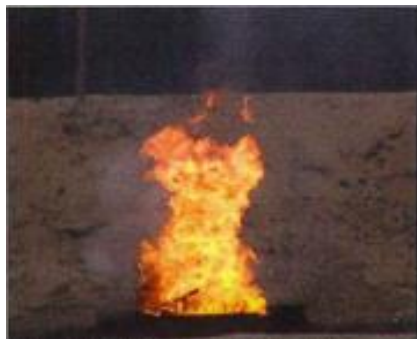
Figure 2: Burning rate test of TFMT-Na in acetone: No fireball / jet / fiery projection
