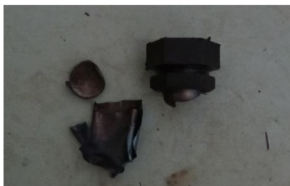
Figure 2: Test tube after the Koenen test (series 1), "F" type
