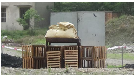
Figure 6: Set-up of the burning test (where wood shavings were inserted between the wood and soaked with kerosene, 7 packages of N-Nitroaminoimidazoline put on metal grid)
