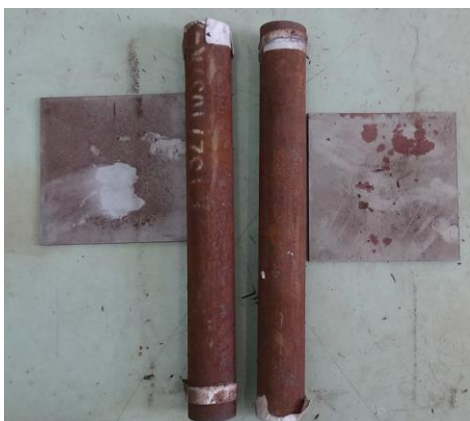
Figure 3: Tube and witness plate after the UN gap test (series 2)
