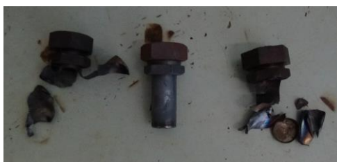
Figure 4: Tube after the Koenen test (series 2)
