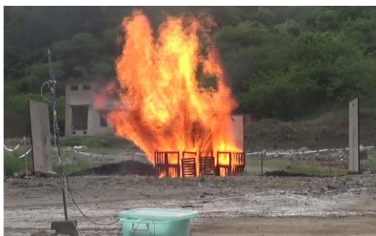
Figure 7 full fire phase (maximum flame) after ignition
