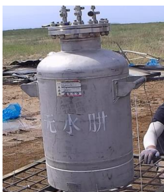
Figure 8: Hydrazine anhydrous packaged in 120 L cylindrical stainless steel storage tank.
