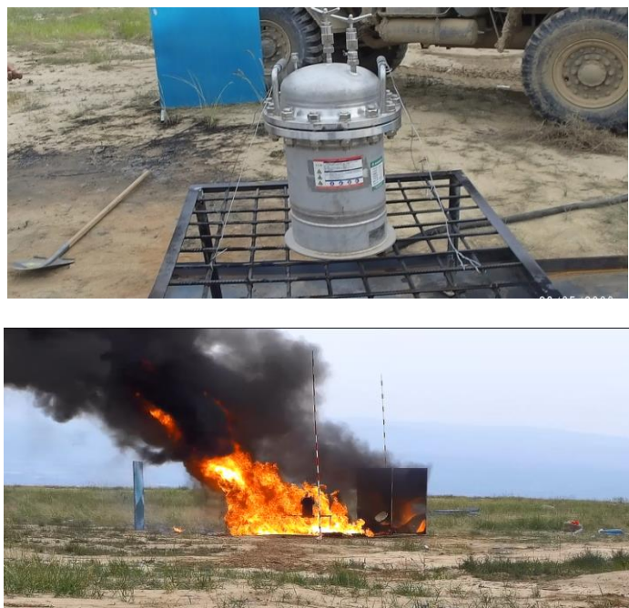
Figure 3: 20 L cylindrical stainless steel storage tank in the 6 (c) test.
