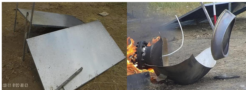
Figure 10: The witness plate and tank after test.
