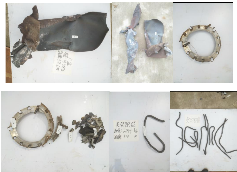
Figure 2: Fragments of the tank after the test.
