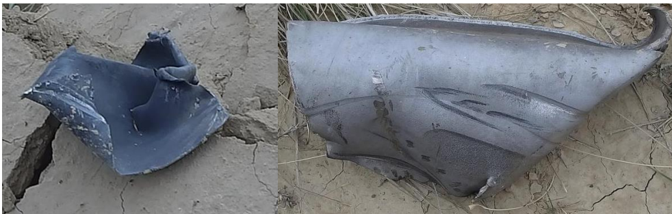
Figure 4: Fragments of the tank after the test.
