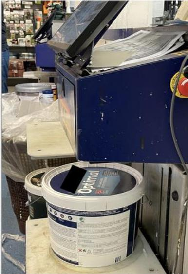
(b) After the tinting process has taken place, the drum is placed in a paint shaker machine (shown below) to mix the various colors into one uniform color.
