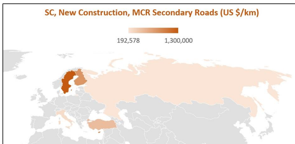
Figure XVIII.5 Single Carriageway Medium Classified Secondary Roads Average New Construction Costs Map (US $/Km) (2016 prices)
