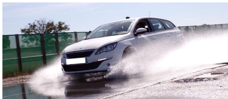
Figure 2.2-8 : Lateral Aquaplaning test method
