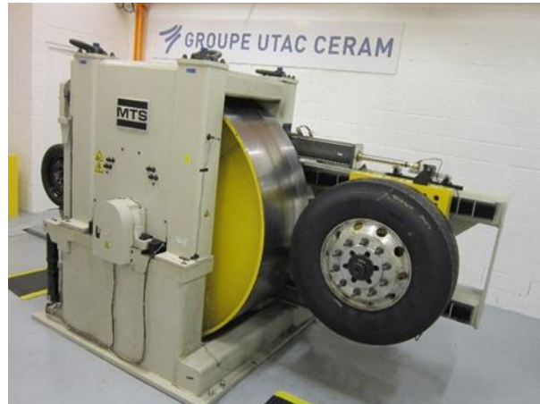
Figure 2.2-1 : UTAC Bench test for Rolling Resistance test
