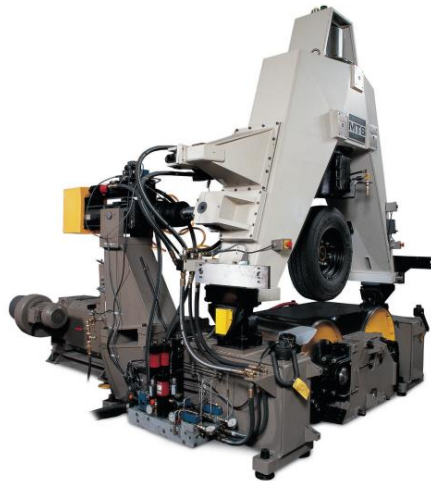
Figure 2.2-5 : Bench test for Flat Trac test
