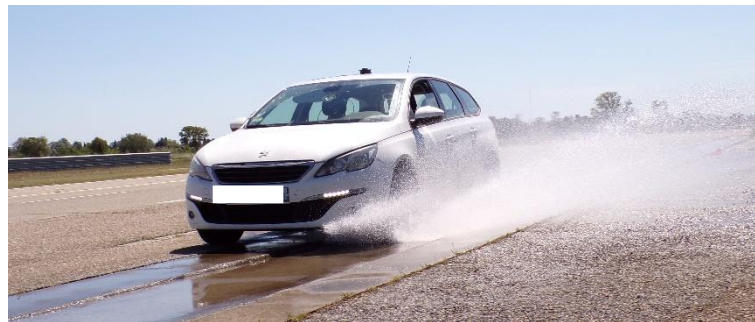
Figure 2.2-7 : Longitudinal Aquaplaning test method
