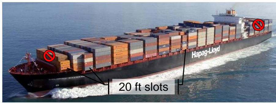
Figure 7 - 20ft container slots
