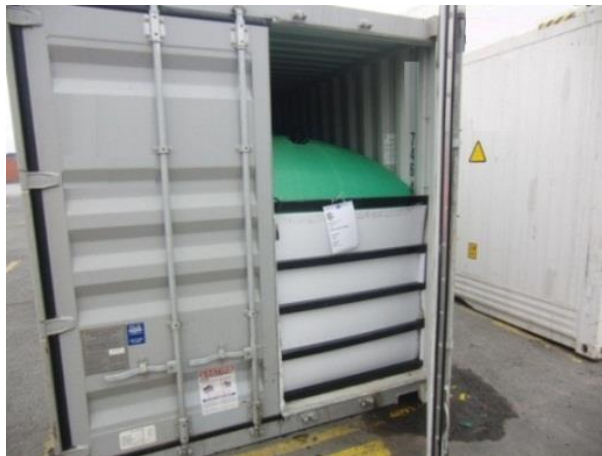
Figure 7.51 Container fitted with flexitank
