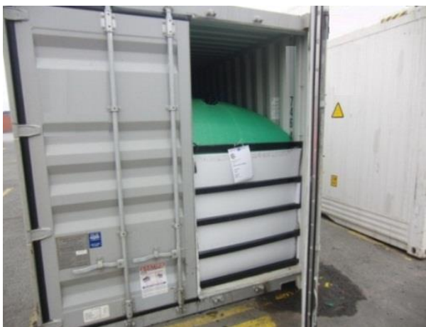
Figure 7.51 Container fitted with flexitank
