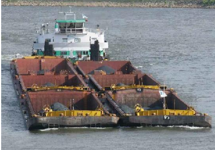
Figure 4 Pushed convoy [photo: Imperial Shipping Holding GmbH, source: BAW 1 ]
