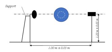
6.4.7. A reference sound, simulating ambient noise emitted by the loudspeaker (see paragraph 6.4.2), equally distributed over the audible reverse warning device as well as the test microphone and measured by the test microphone (Figure 2 in Annex 4), shall emit pink noise at three different sound pressure levels. The reference sound level for:
