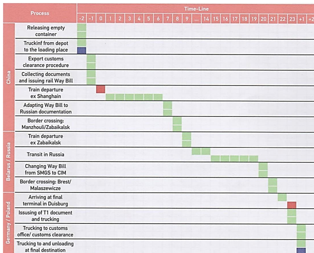
Figure 16 FELB Technology of Container transport between China and Europe / Procedures and Documentation needed
