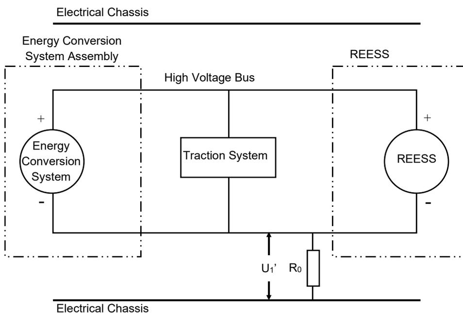
If  $U_2$  is greater than  $U_1$ , insert a standard known resistance ( $R_0$ ) between the positive side of the high voltage bus and the electrical chassis. With  $R_0$  installed, measure the voltage ( $U_2'$ ) between the positive side of the high voltage bus and the electrical chassis (see Figure 6 below). The electrical isolation ( $R_i$ ) is calculated according to the following formula:
