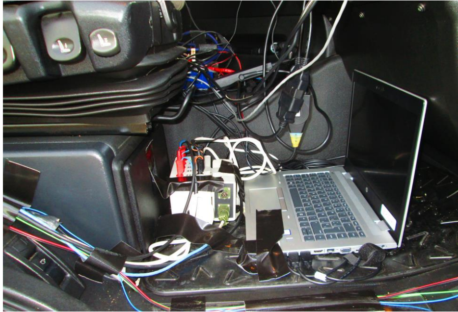
Figure 37 INCA devices, OBD connectors, analyzer and laptops used
