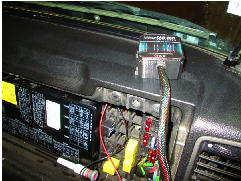
Figure 35 Urea emulator installed in the vehicle
