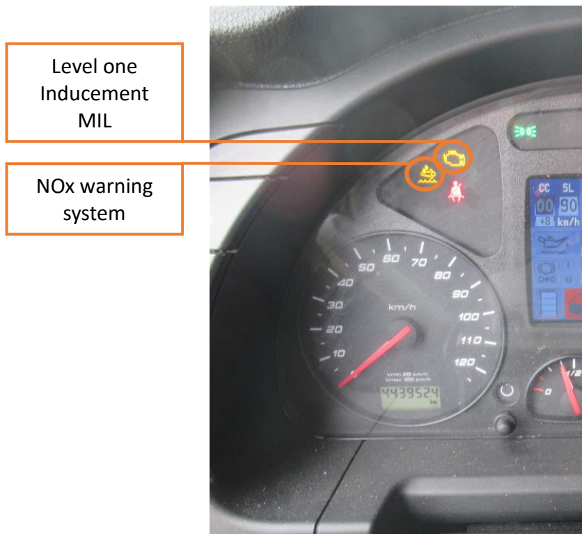
Figure 9 Vehicle's cluster with MILs and warnings.
