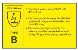
(d) In addition, when appropriate, our members already use a label on composite IBCs providing supplementary information. A new standard is currently being developed (IEC 61340-4-11 Electrostatics – Part 4-11: Standard test methods for specific applications – Testing of electrostatic properties of composite IBC) that will include the label also e.g.:
