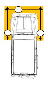
$\Phi$ 0.3m×1.0m pole 0.3m \*5 years old child Center of side mirror (UN-R46 class III) 0.3m
