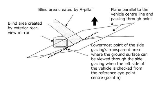
The range of the blind area created by the A-pillar or exterior rear-view mirror in paragraph 15.2.4.10. shall be an area that meets the following formula. In this case, if there are more than one blind area, each blind area shall meet the conditions of the formulae.
