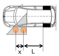
If Ls<=L, vehicle can stop before run over by rear wheel.
