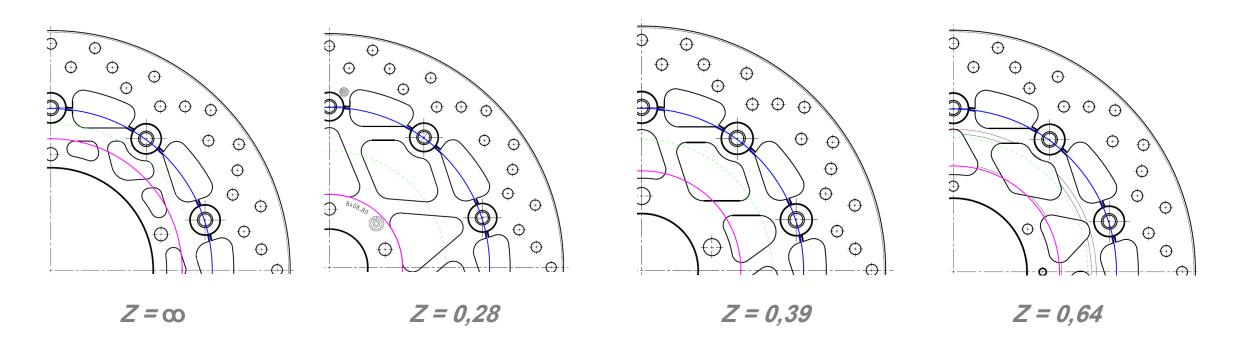
By applying the proposed modification the calculation is related only to the bell characteristics (no influence of braking surface geometry on the results) and gives a more balanced output.
