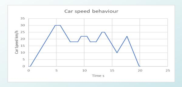
Vehicle speed simulation based on real driving
