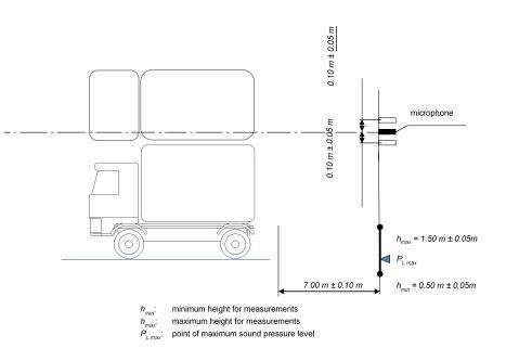
14.2.2.1. "Non-self-adjusting audible reverse warning device" or "Multiple audible reverse warning system" shall emit sound:
