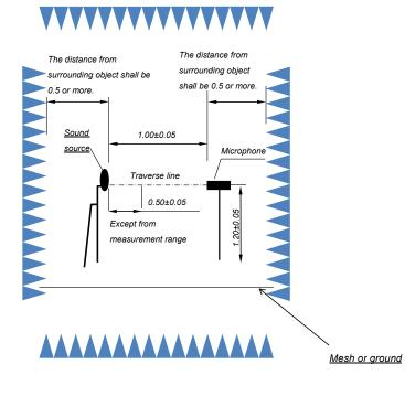
6.3.7. Under the conditions set forth above, the A-weighted sound pressure level shall comply with the following for "Non-self-adjusting audible reverse warning device" or "Multiple audible reverse warning systems":
