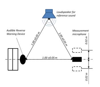
6.4.7. A reference sound, simulating ambient noise emitted by the loudspeaker, equally distributed over the audible reverse warning device as well as the test microphone and measured by the test microphone (Figure 1), has to emit pink noise at three different sound pressure levels. The reference sound loudspeaker shall be at the same height as the device and the measurement microphone. The reference sound for:
