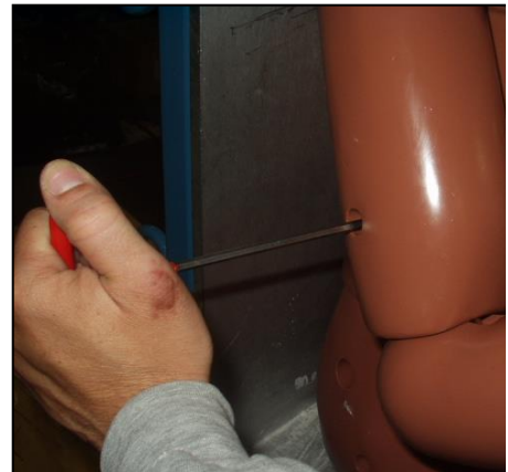
Figure 61 Access hole for the elbow rotation bolt
