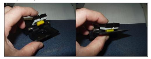
Remove the two M2.5 SHCS that retain the T1 pin at the C7-T1 joint (Figure 82). Slide the T1 pin out of the vertebrae joint (Figure 83) and set it aside along with the two M2.5- $0.45 \times 8$  SHCS for re-installation later."
