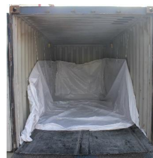
Figure 35: Half height liner
