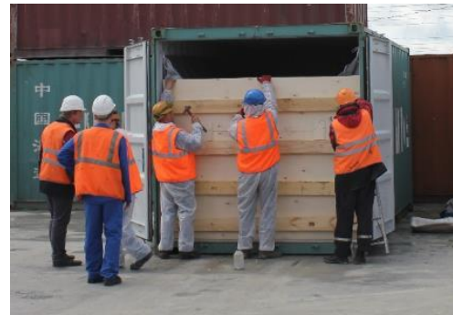
Figure 50 Rear false bulkhead
