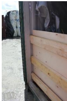
Figure 49 Use of shoring slots
