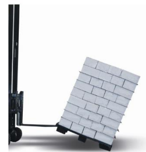
Figure 28 - With anti-slip sheets
