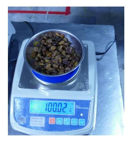
3.5 Size of the reduced sample (analytical sample) (2) The reduced sample is taken from the composite sample and must comprise at least 100 g in case of dried grapes.
