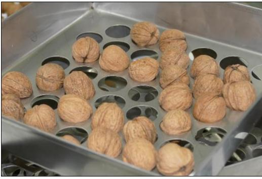
3.6.4 Verification of the size (2) Illustration: The reduced sample is shaken and the number of nuts meeting the size of the respective sieve is determined.
