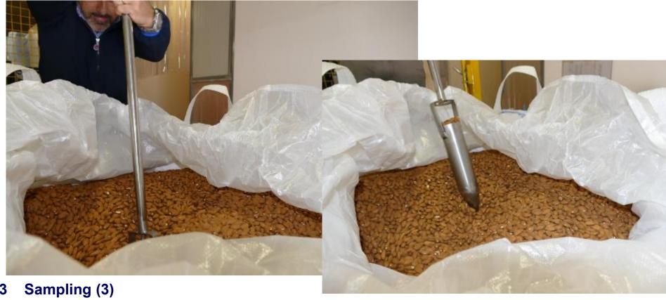
A conformity check shall be made by assessing bulk or composite samples. It is based on the principle that the quality of the randomly taken samples is representative of the quality of the lot.
