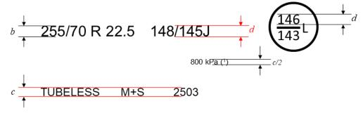
(1) PSI marking instead of kPa is allowed for tyres first type approved before 1 January 2018. The kPa marking may be preceded by "TEST AT:" or, alternatively, by "TEST INFL:" or the symbol "@".
