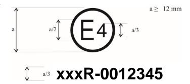
The above approval mark, affixed to a tyre shows that a tyre concerned has been approved in the Netherlands (E 4) pursuant to UN Regulation No. [xxx], under approval number 0012345. The first two digits of the approval number (00) indicate that the approval was granted according to the requirements 00 series of amendments to this Regulation.
