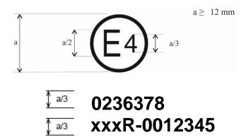
The above approval mark (according to paragraph 5.5. of this Regulation) shows that the tyre concerned has been approved in the Netherlands (E 4) pursuant to UN Regulations Nos. 30 and [xxx]. The first two digits of the approval numbers indicate that, at the dates when the respective approvals were granted, UN Regulation No. 30 included the 02 series of amendments while UN Regulation No. [xxx] was in its original form.
