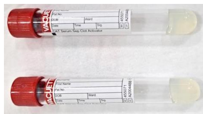
Figure 7: Primary receptacle. Non-pressure test-resistant tube without screw tap. (Source: Testing laboratory AIDIMME)
