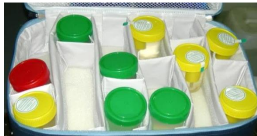
Figure 6: Primary receptacle. Non-pressure test-resistant tube with screw tap without sealing ring. (Source: Testing laboratory AIDIMME)
