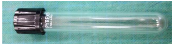
Figure 5: Primary receptacle. Pressure test resistant glass tube with screw tap and sealing ring. (Source: Testing laboratory AIDIMME)
