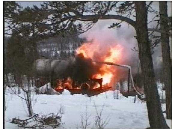
Figure 1-2: The tank during fire. White smoke indicates decomposing emulsion matrix.
