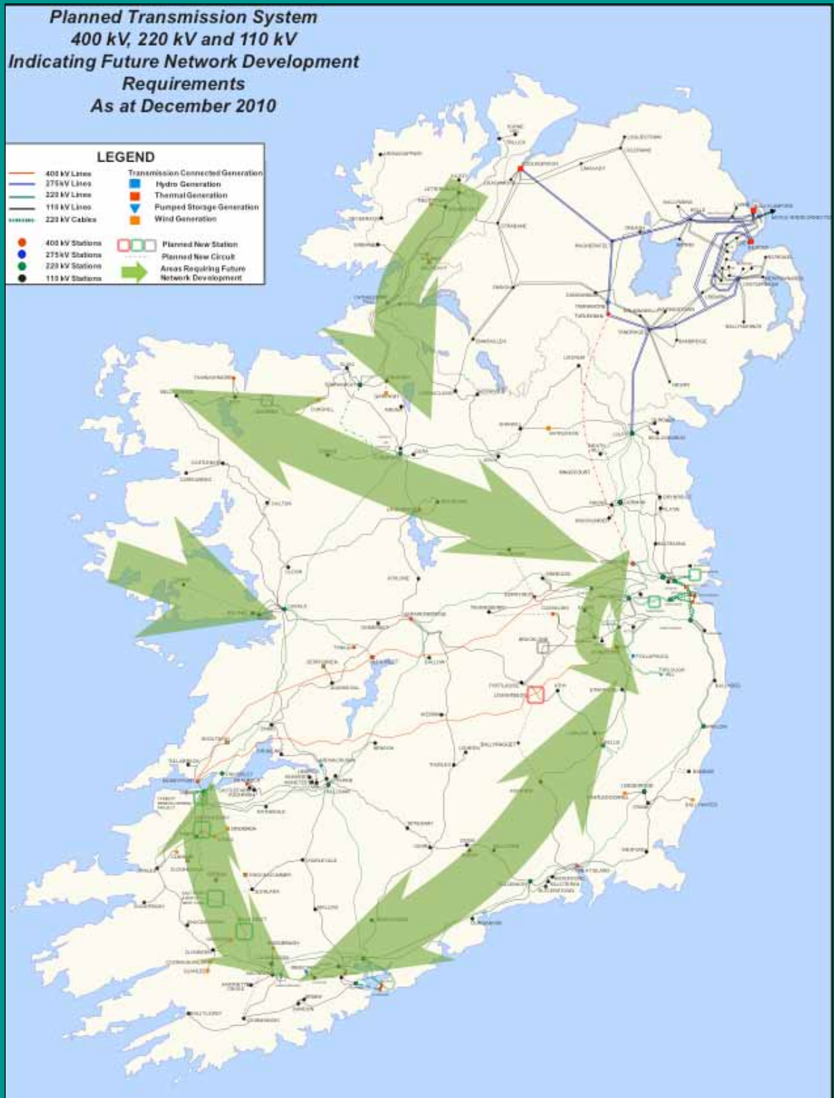
Figure 2.3 Map Indicating Future Network Development Requirements (extract from EirGrid Transmission Development Plan 2010)
