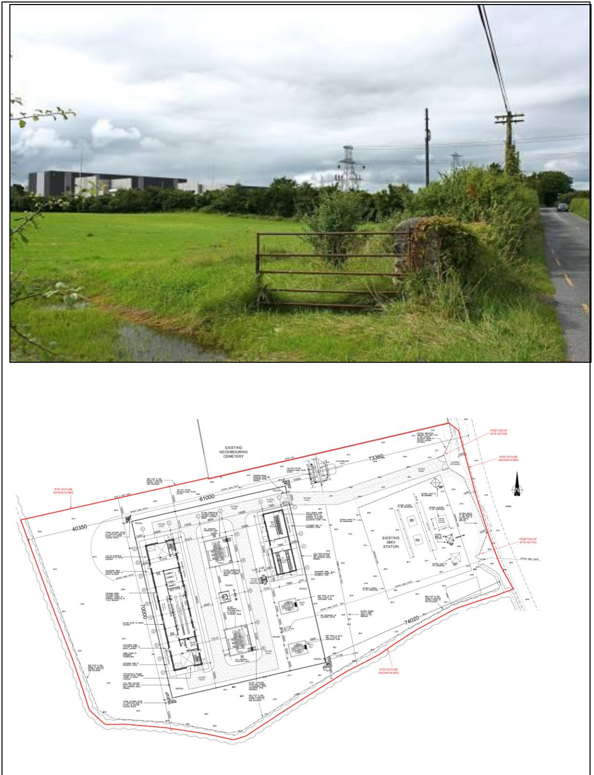
Figure 8.5: Photomontage and Site Layout of the Proposed Ballyragget 110 kV/38 kV/ MV substation
