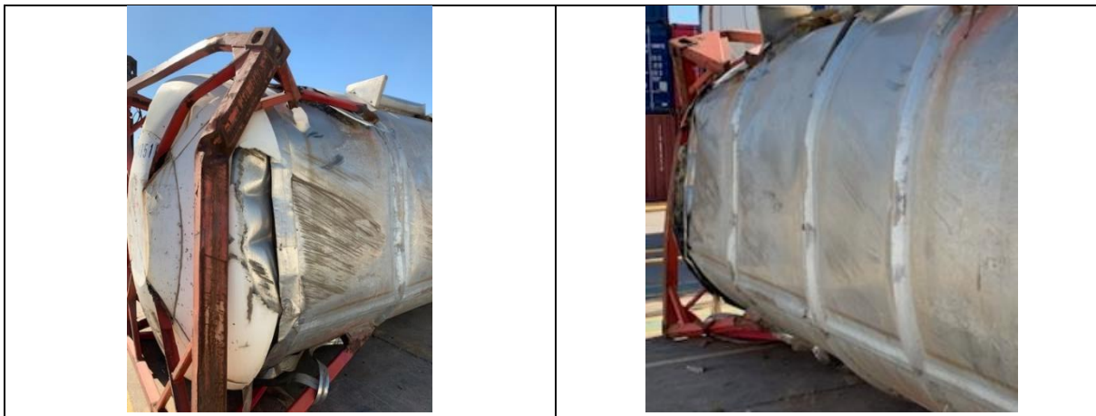
Portable tank container damage following overturn accident: Note the absence of penetrating tears in pressure envelope.
