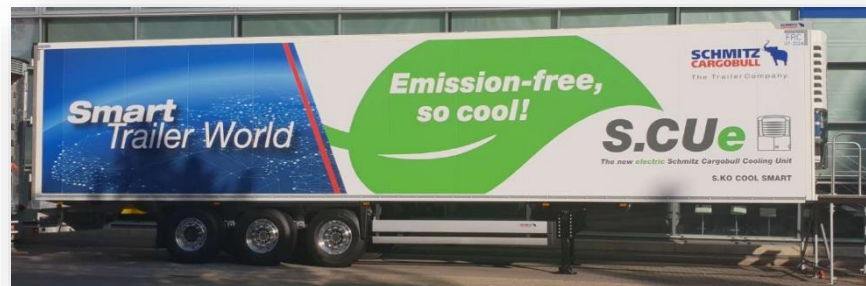
Schmitz Cargobull – Electrified cooling unit with energy provided by trailer axles
