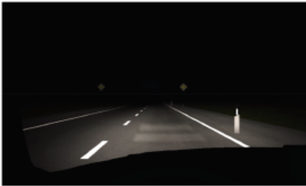
Figure 5: Picture of two lines transverse to the driving direction in positive contrast on standard low beam that was shown to the test subjects in the simulative study.
