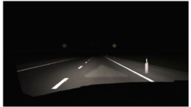
Figure 2: Picture of a triangle in positive contrast on top of a common low beam that was shown to the test subjects in the simulative study.
