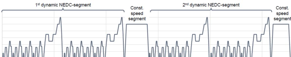
The dynamic NEDC segments DS<sub>1</sub> and DS<sub>2</sub> are used to calculate the electric energy consumption. The constant speed segments CSS<sub>M</sub> and CSS<sub>E</sub> are intended to reduce test duration by depleting the REESS more rapidly than driving consecutively NEDC test cycles.
