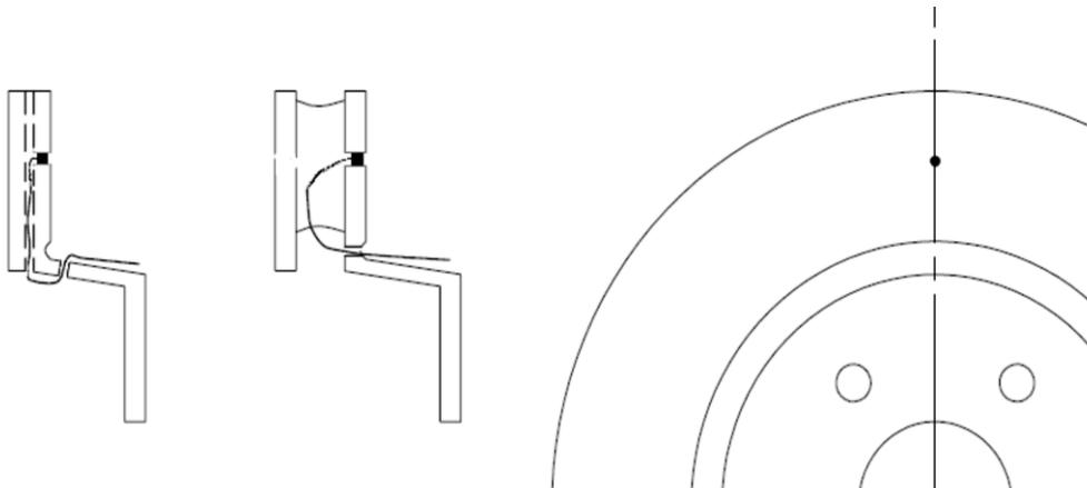
NOTE 1 — Optional — For brake pads, embed one thermocouple at a depth of 2.0 mm near the centre of the friction surface on each pad. For disc brake pads with grooves, install the thermocouple at least 4.0 mm from the groove edge on the leading side of the pad. For inboard pads on single-piston callipers, install the thermocouple on the leading edge, 3.0 to 4.0 mm from the piston outside diameter near the centre of the friction surface.
