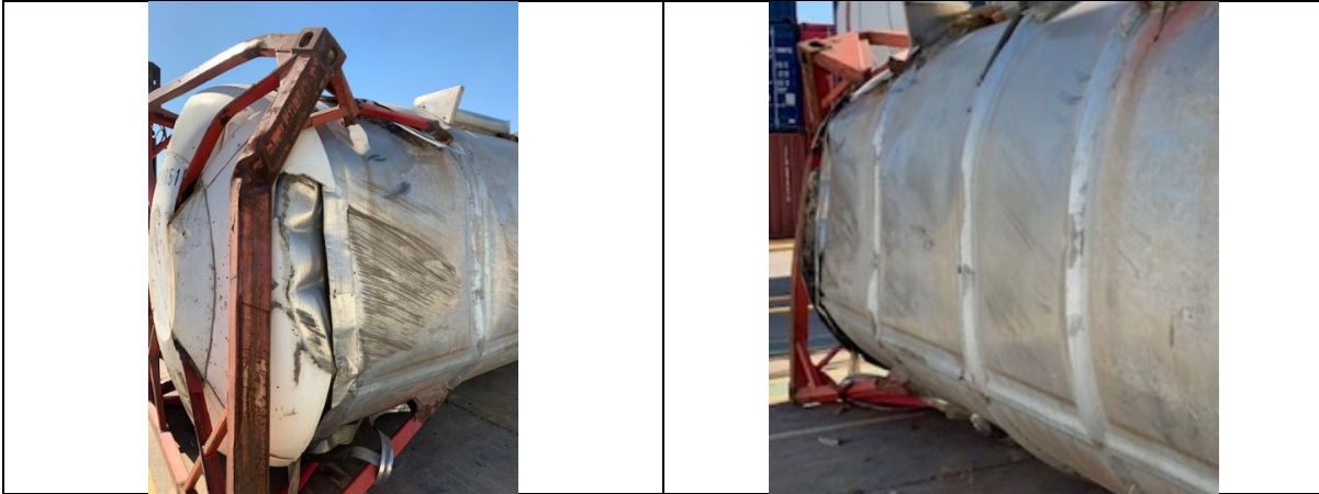
Portable tank container damage following overturn accident: Note absence of penetrating tears in pressure envelope.
