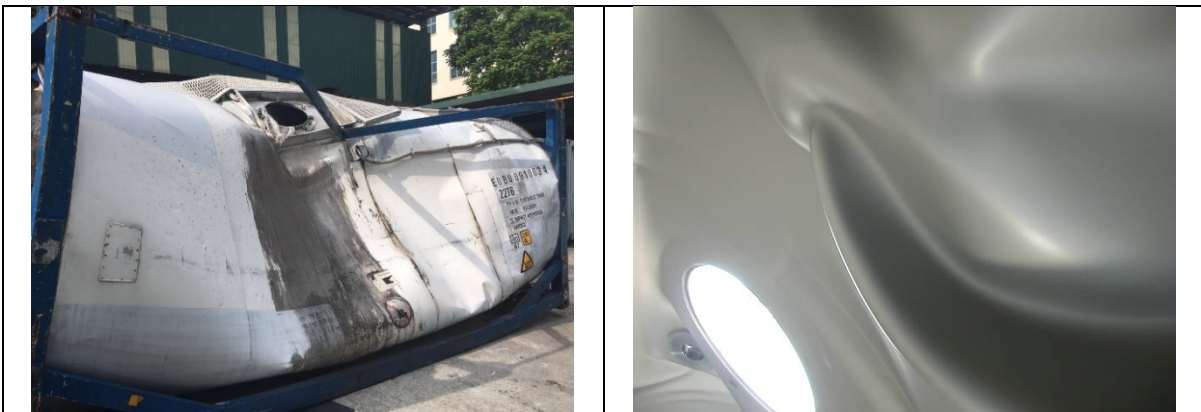
Portable tank container suffered impact in handling accident. Note minimal protection from ISO frame – energy absorbed without fracture of shell.
