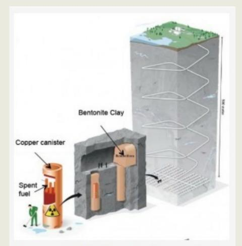
The so-called KBS-3 method, suggested in Sweden in the 1980s, proposes placing spent fuel inside hermetically sealed copper canisters in a bentonite clay environment in crystalline bedrock at a depth of 500 meters. (Source: mkg.se.)
