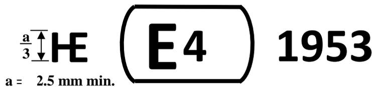
The approval mark above affixed to the light source, preceded by the character “HE”, indicates a high-efficiency LED replacement light source that has been approved in the Netherlands (E 4) under the approval code 1953.
