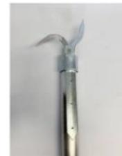
The boat’s hook is used to be able to get ropes and steel cables on f.a. bollards or “duck dalves” which are not easy reachable. It prevents crew members to climb on objects and enables them to stay on board (working safety).
