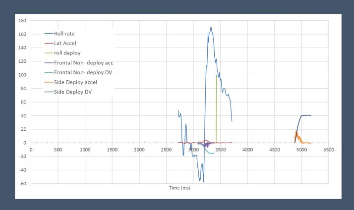
Requiring all parameters to be recorded in all event triggers means data cannot be stored to non-volatile memory until the roll ends (in this case 11.765 seconds). Events may not be recorded while waiting for this event to complete. However, with tailored EDR, the data is recorded as each event occurs
