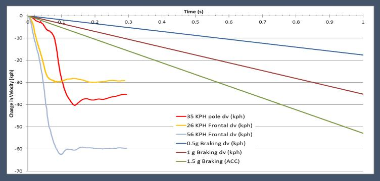
The delta-V in longitudinal crashes typically peaks about 0.1 to 0.15 seconds after contact. The other plots are delta-V from various fixed braking deceleration levels.
