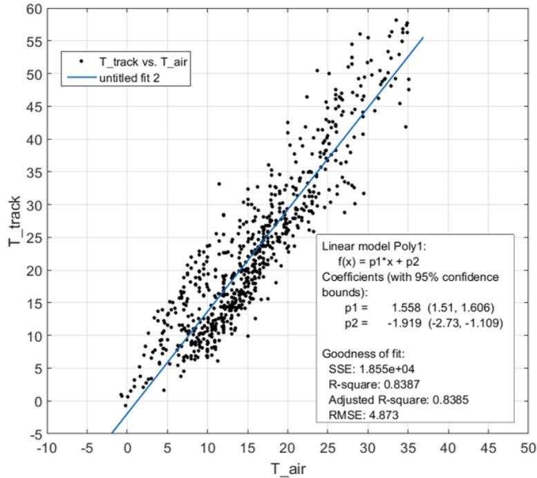
Measurements of air and track surface temperature (about 700) measurement points under various ambient conditions (summer, winter, cloudy, sunny, etc...)
