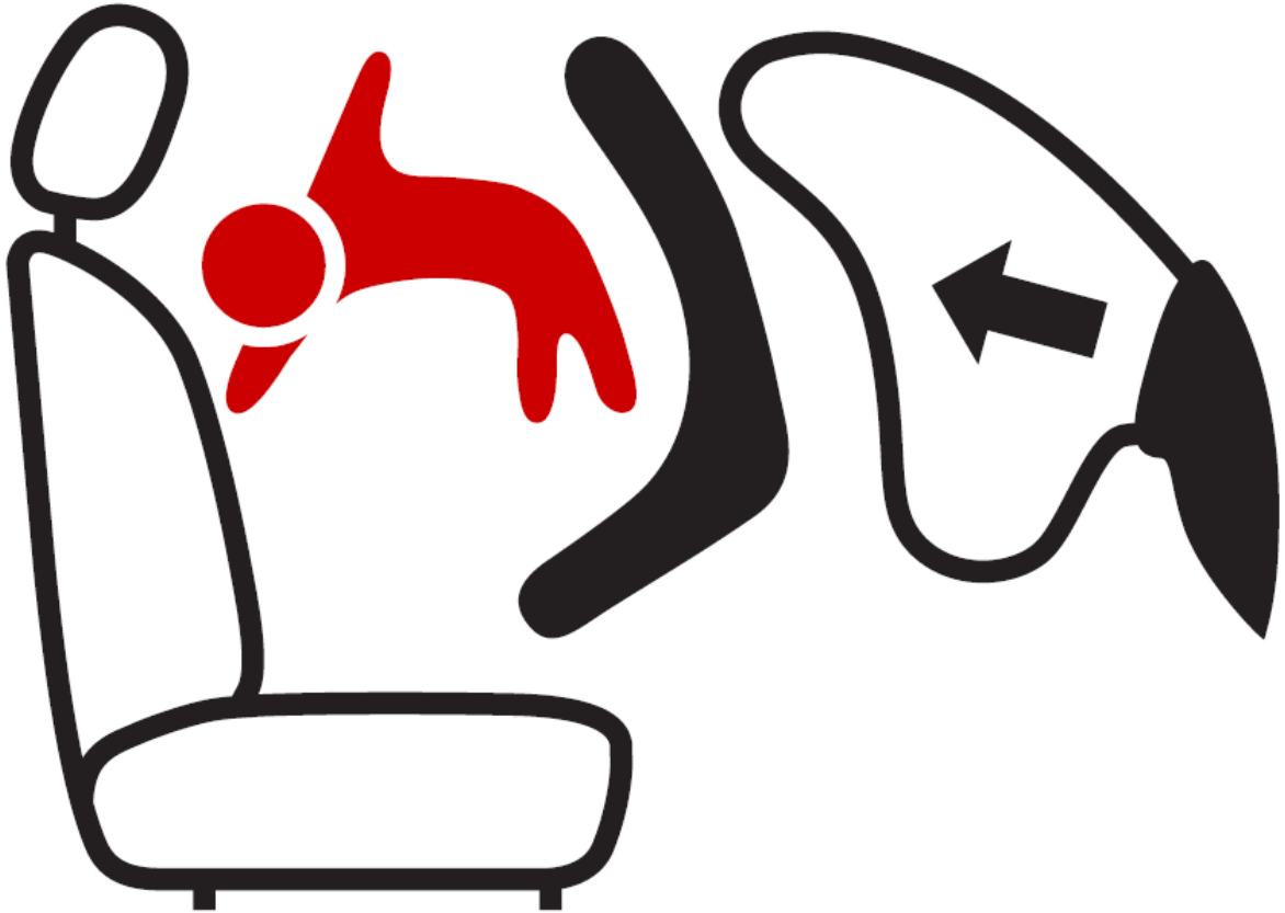
Figure C Pictogram depicting airbag deployment danger that shall be used and that shall measure 40 mm in width and 28 mm in height or proportionally larger
