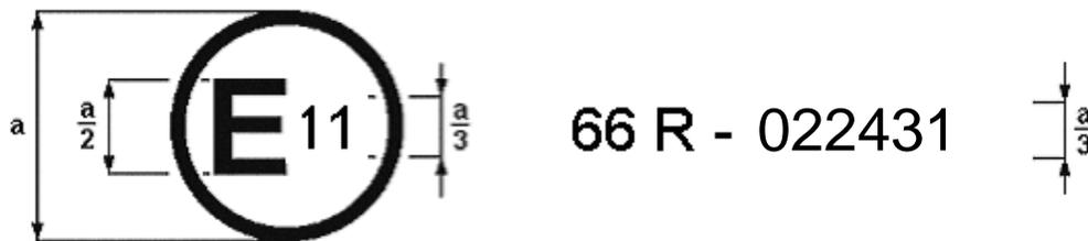
The above approval mark affixed to a vehicle shows that the vehicle type concerned has, with regard to the strength of the superstructure, been approved in the United Kingdom (E11) pursuant to Regulation No. 66 under approval number 022431. The first two digits of the approval number indicate that the approval was granted in accordance with the requirements of the 02 series of amendments to Regulation No. 66.”
