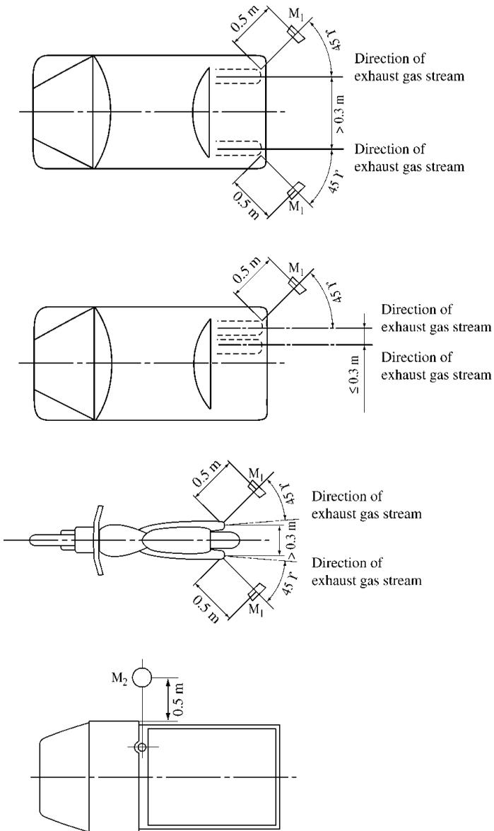
Case where the outlet of exhaust pipe is directed upwards
