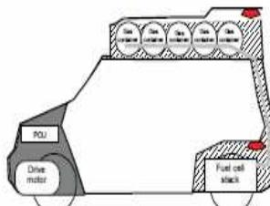
Example 4. Hydrogen system components installed at the roof and under the floor of the body
