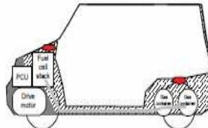
Example 1. Hydrogen system components installed in the motor room and under the floor of the body
