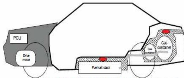
Example 7. Hydrogen system components installed under the floor of the body and in the housing in the luggage compartment
