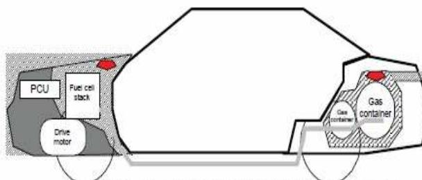
Example 6. Hydrogen system components installed in the motor room and in the housing in the luggage compartment
