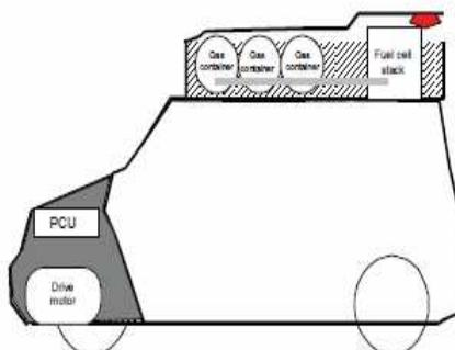
Example 5. Hydrogen system components installed at the roof
