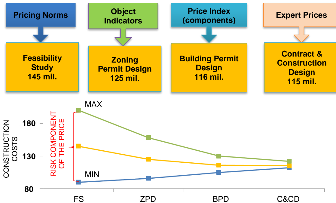
Figure V Increasing accuracy of construction costs during construction preparation with inclusion of the risk component of the prices)
