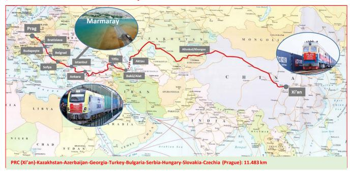
"China Railway Express" block container freight train which was 850 meters long, comprised of 42 wagons loaded with high-cube containers and carrying electronic components, was dispatched from Xi'an, China and arrived in Prague, Czechia via Iron Silk Road through Kazakhstan, Azerbaijan, Georgia using the Marmaray tunnel.
